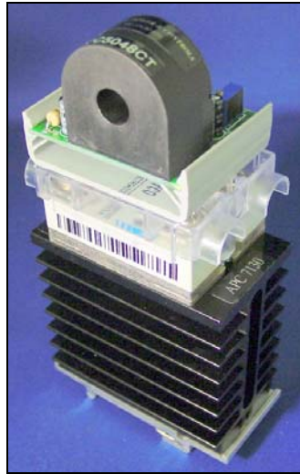
APC7130 SSR Assembly w/ APC5048CT Mounted
