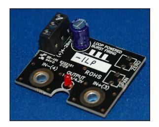
The APCMAN-1LP is designed for use in a broad range of 4 to 20mA power control applications where an external power supply is not available. The APCMAN-1LP mounts directly on the input connections of a Solid State Relay (SSR) and provides precise 0-100% time proportioned drive based on the input signal.
